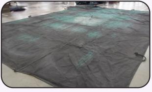
WEAVE DISINTEGRATION, DRY-ROTTING, ETC.
